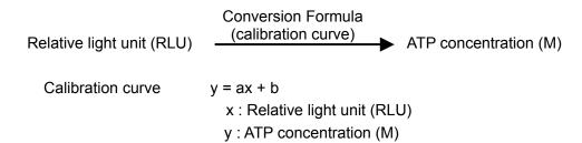
Relative light unit (RLU) can be converted to ATP concentration by entering "a" and "b" beforehand.
