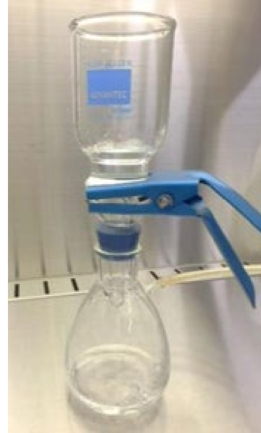
Membrane filtration assembly: Funnel + Locking ring + Flask + etc.
