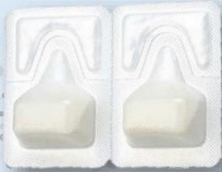
To detect and quantify the presence of Total Coliforms and Fecal Coliforms (Escherichia coli in water)
